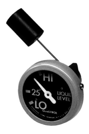
A magnetic liquid level gage is used to indicate the level of the insulating liquid in the main transformer tank and in associated compartments. It consists of a two piece assembly. One piece contains the float arm, a magnet and the flange for sealing to the tank. The other piece contains the gage itself with a magnetically operated pointer.
