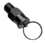
A manual/automatic pressure relief valve is normally supplied on all liquid filled transformers. The valve is supplied with a manual pull ring which can be used to vent the transformer to the atmosphere before being placed in service or to manually relieve the internal tank pressure. The valve will also operate automatically at 10 psi to relieve excessive pressure in the tank.
