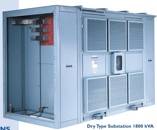
Primary 6.3kVΔ Secondary 400Y/23 IV 50Hz; I50°C Rise; Copper Wound; Digital Temperature Monitor; NEMA 3R Louvers; Low Voltage Transition Section with Flex Leads
