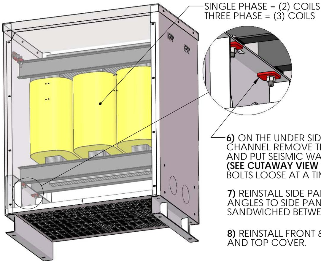
6) ON THE UNDER SIDE OF THE MOUNTING CHANNEL REMOVE THE ROUND WASHERS AND PUT SEISMIC WASHERS IN THEIR PLACE. (SEE CUTAWAY VIEW 2) NO MORE THAN 2 BOLTS LOOSE AT A TIME. (QTY. 4)
