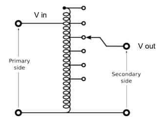
As explained by the figure, an auto transformer has the capability to supply a varying secondary voltage to the externally connected load. So this is mostly used in applications where various voltage outputs is required. Some of its applications are listed below:
